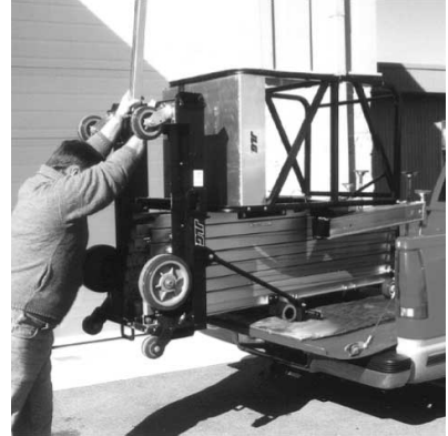
Figure 14. Loading Machine onto Bed of Pick-Up Truck.
