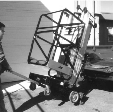
Figure 14. Loading Machine onto Bed of Pick-Up Truck.
